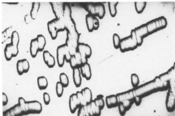
Figure 2 A \{001\} surface showing elevated structures at isolated sites and in arrays ( \times 118 ).
